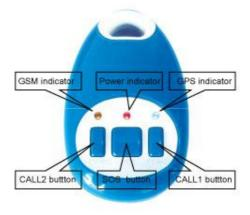
Press the on/off button for 5 second outdoors to start the tracker. Three LEDs will be bright at the same time during the tracker starting. In 10 to 30seconds, the unit will begin to work and indicators will blink as the following:
